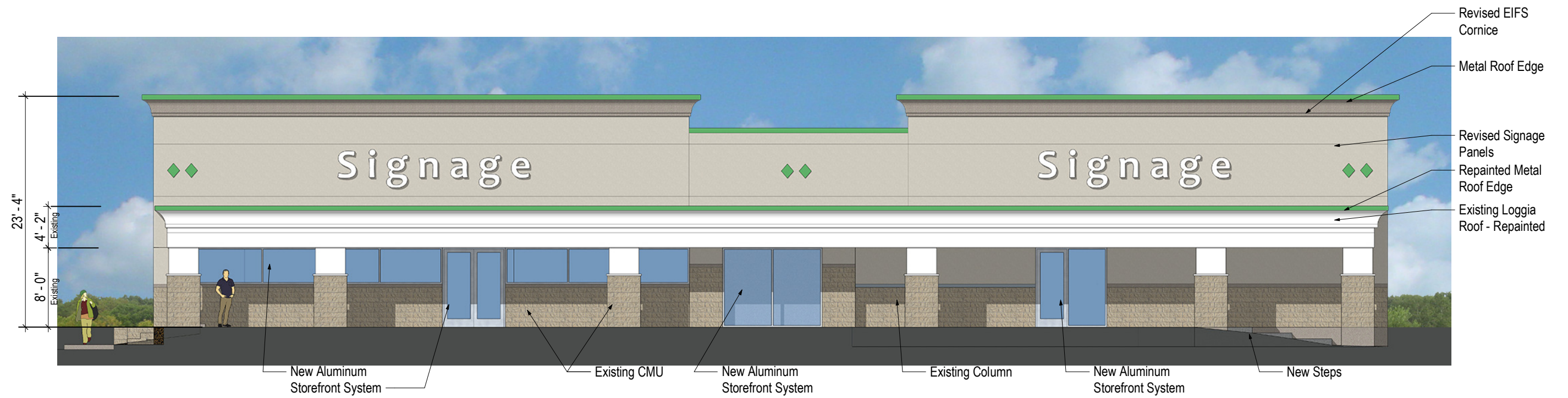
② Renovated Main St. Elevation 3/16" = 1'-0"
